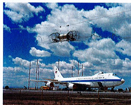
EMP simulator HAGII-C testing a Boeing E-4 aircraft.
