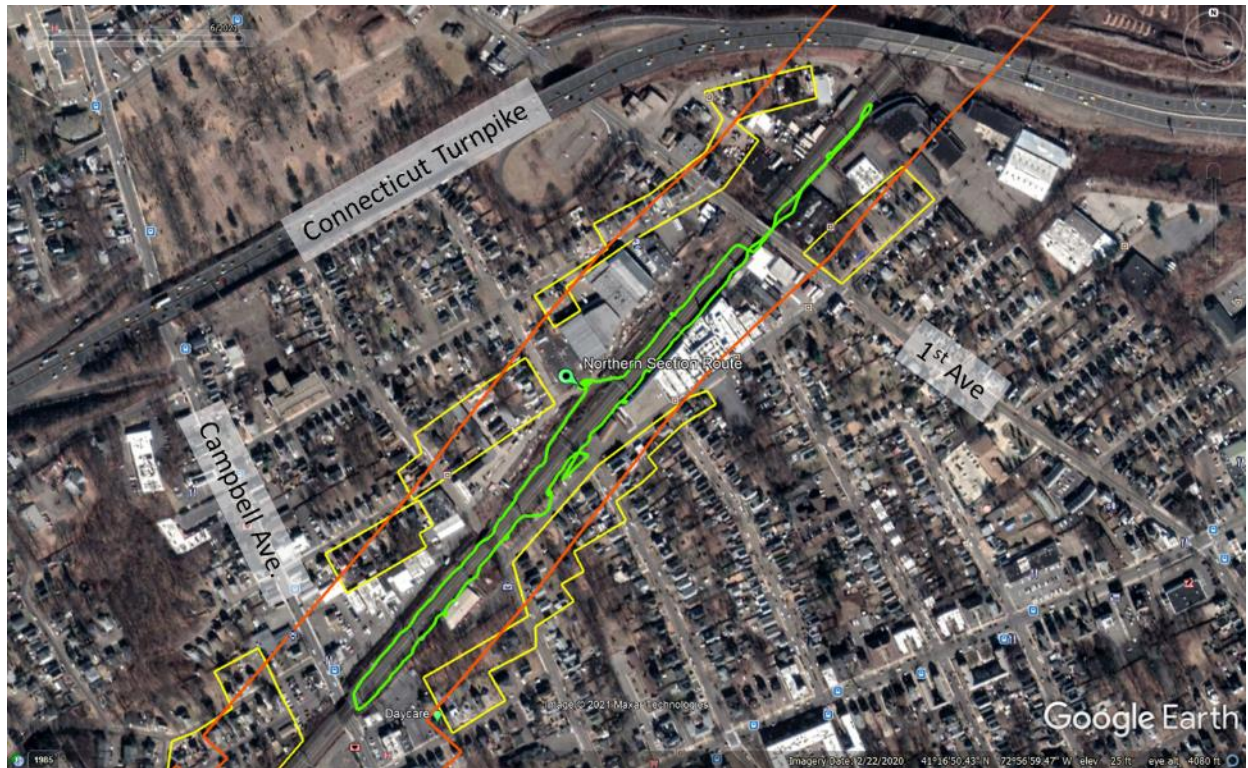
Figure D-2. EMF measurements were obtained along approximately 0.6 miles of the northern portion of the proposed route (in West Haven) and on both sides of the CT DOT corridor where possible. The green trace provides the GPS-tracked measurement path.
