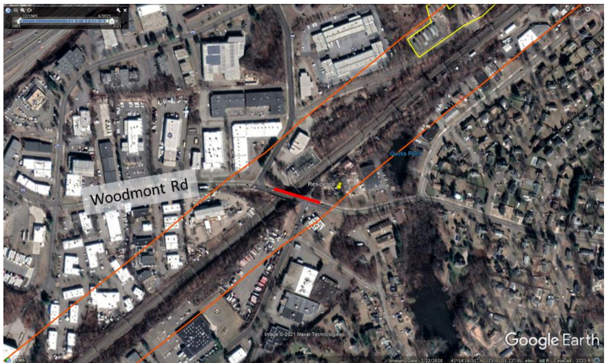
Figure D-15. EMF measurements were obtained along the Woodmont Road overpass (in Milford) and used to generate the transect profile. Orange lines show the distance of 300 feet from the proposed transmission line.
