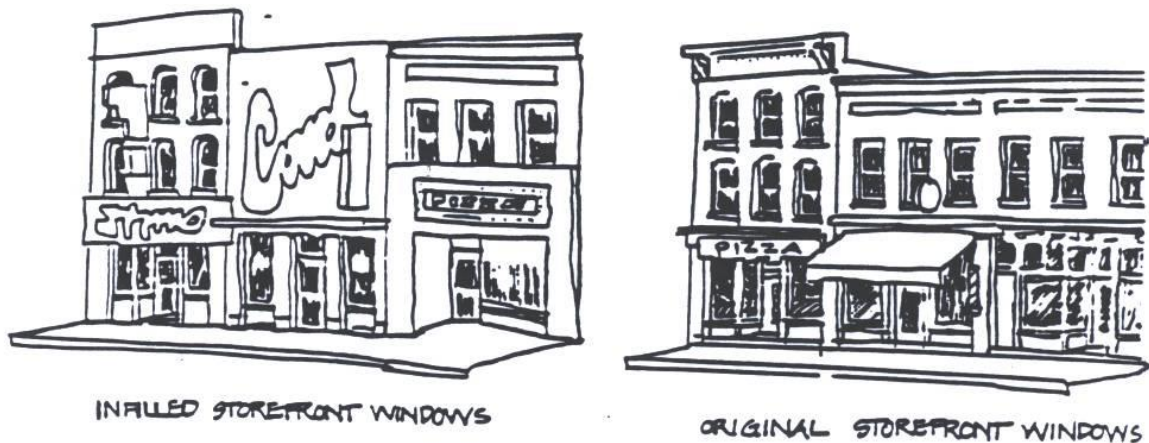
Illustration 20.2 Avoid Attempts at Hiding an Older Façade.
