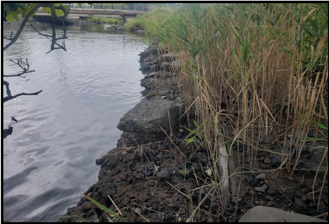
Photo 15: Urban derived Udorthent soil in southwestern portion of Indian River survey area. Note large pieces of asphalt. Photo taken looking south. 9/16/2021.
