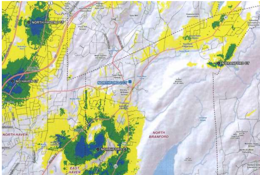
Figure 4 – Cellco Existing 2100 MHz coverage
