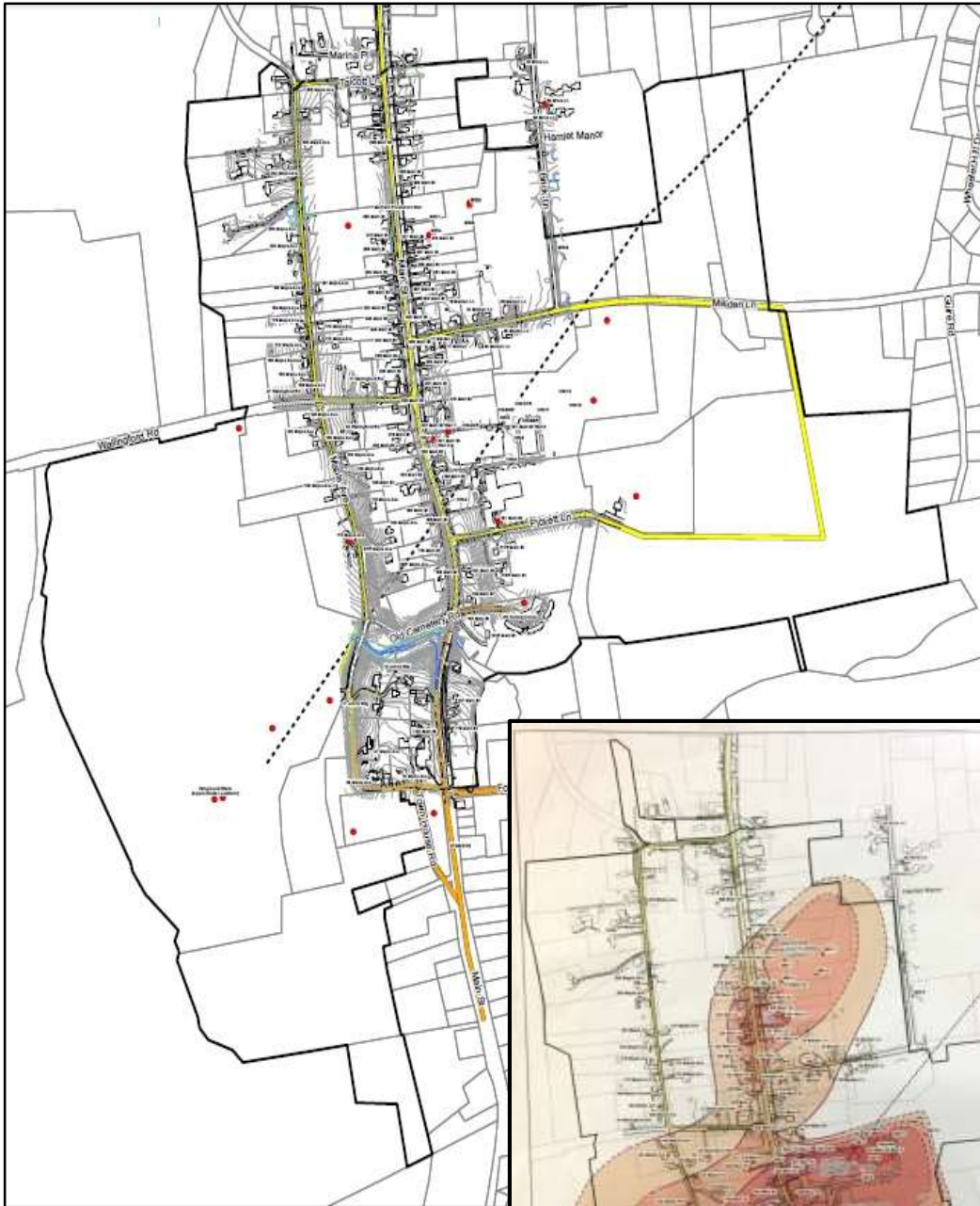
Durham Groundwater Management Zone (above) and area of trichloroethylene (TCE) contamination (inset)
