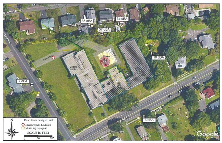
Figure 6: Graphical Summary of the Modeling Results Under Worst-Case Nighttime Operating Conditions (Cooler)
