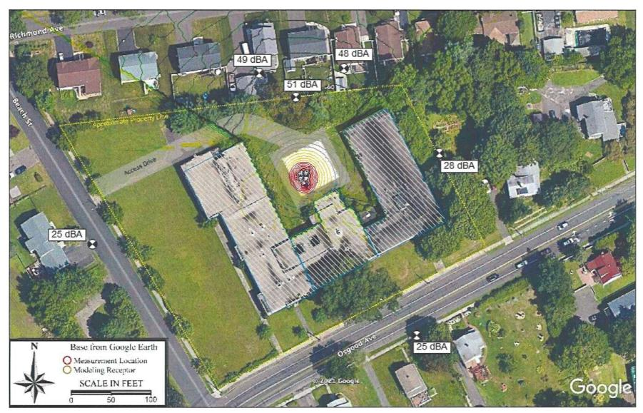
Figure 5: Graphical Summary of the Modeling Results under Worst-Case Daytime Operating Conditions (Gen + Cooler)
