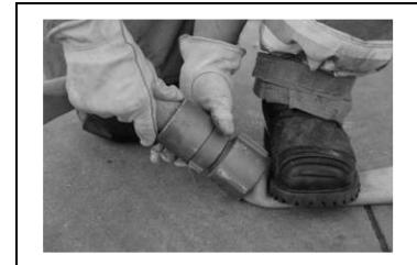
**One-Fire Fighter Knee-Press Method of Uncoupling a Fire Hose**
