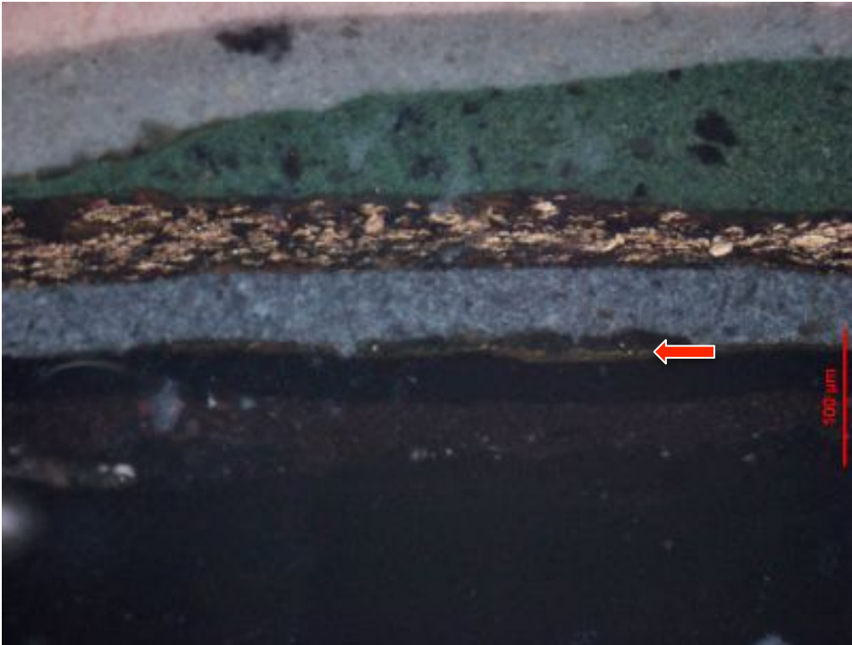
Figure B4c: Cross Section, Sample B, door grill palmette, brightfield, 200x magnification. Red arrow indicates location of original metal leaf finish.
