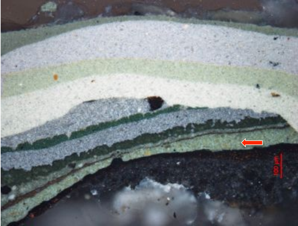
Figure B8a: Cross Section, Sample L, spandrel panel, brightfield, 100x magnification. Red arrow indicates the location of the original, medium green finish.
