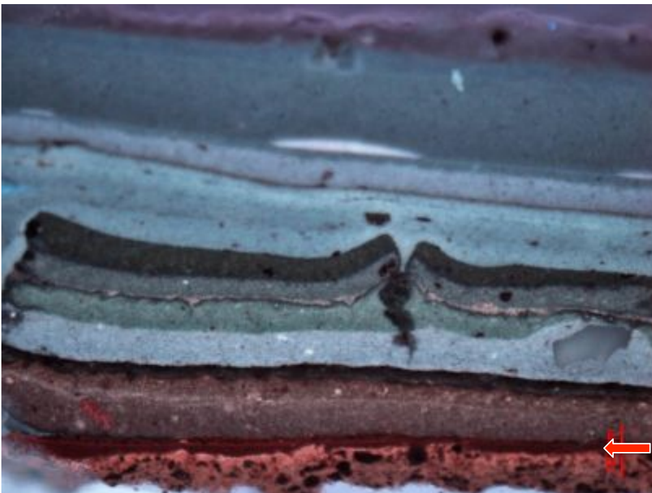
Figure B1b: Cross Section, Sample A, door grill frame, ultraviolet light, 100x magnification. Red arrow indicates the location of the original, deep black finish.
