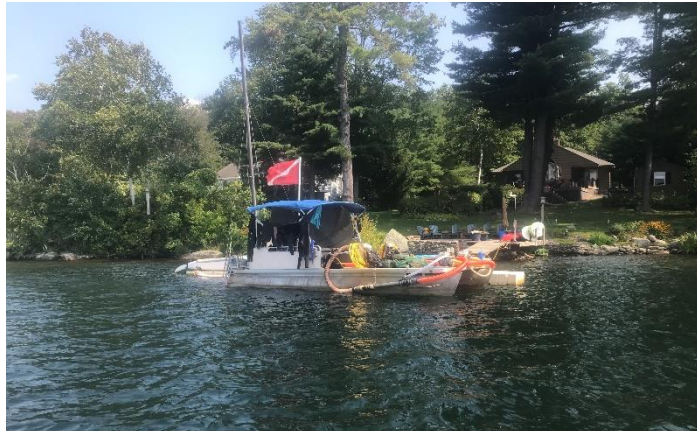
Figure 3. Diver assisted suction harvesting apparatus used during the CAES IAPP 2022 survey.
