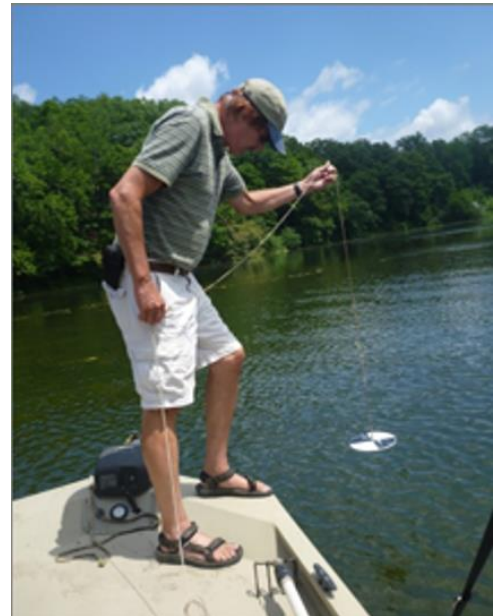
Figure 3. Checking water clarity with Secchi disk.
