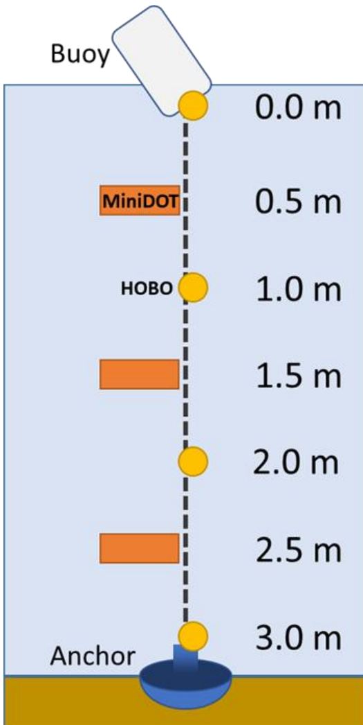
FIGURE 3. Example of a datalogging buoy, though instrumentation and depths vary. In Gardner, the top of the buoy remained submerged, was anchored at 12 m depth, and had three miniDOTs at 10, 6, and 2 m deep.
