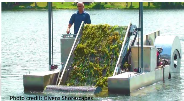
Figure 9. Eco-Harvester technology may improve removal of plant roots.
