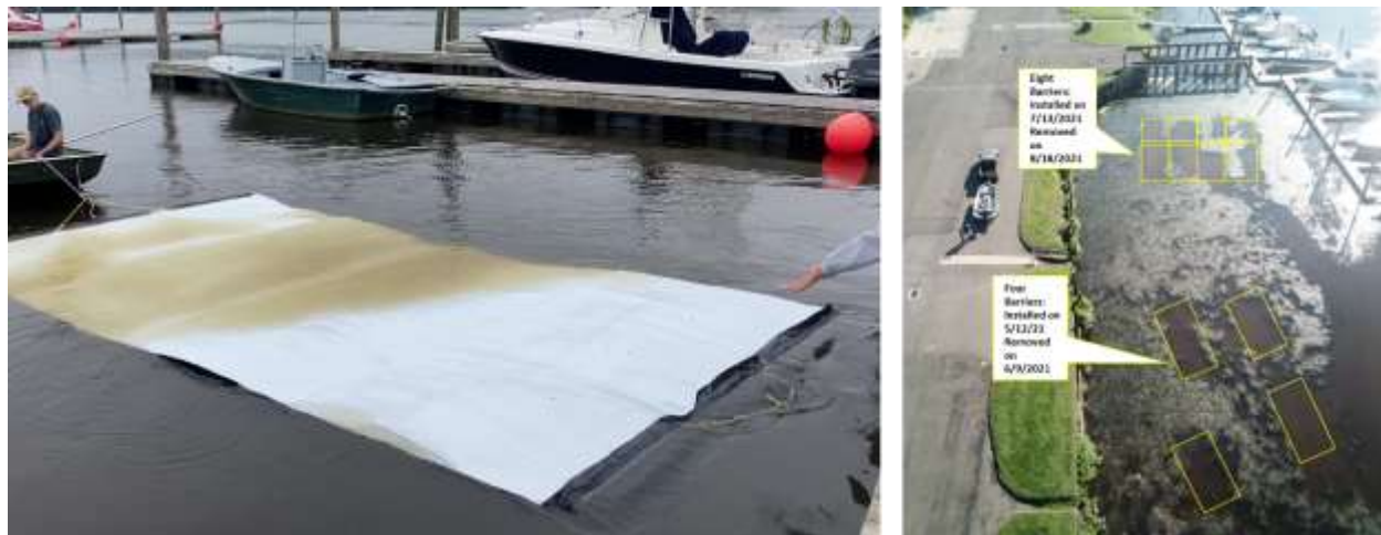
Figure 16. CAES IAPP testing of short-term benthic barriers on the Connecticut River at Portland Boat Works.
