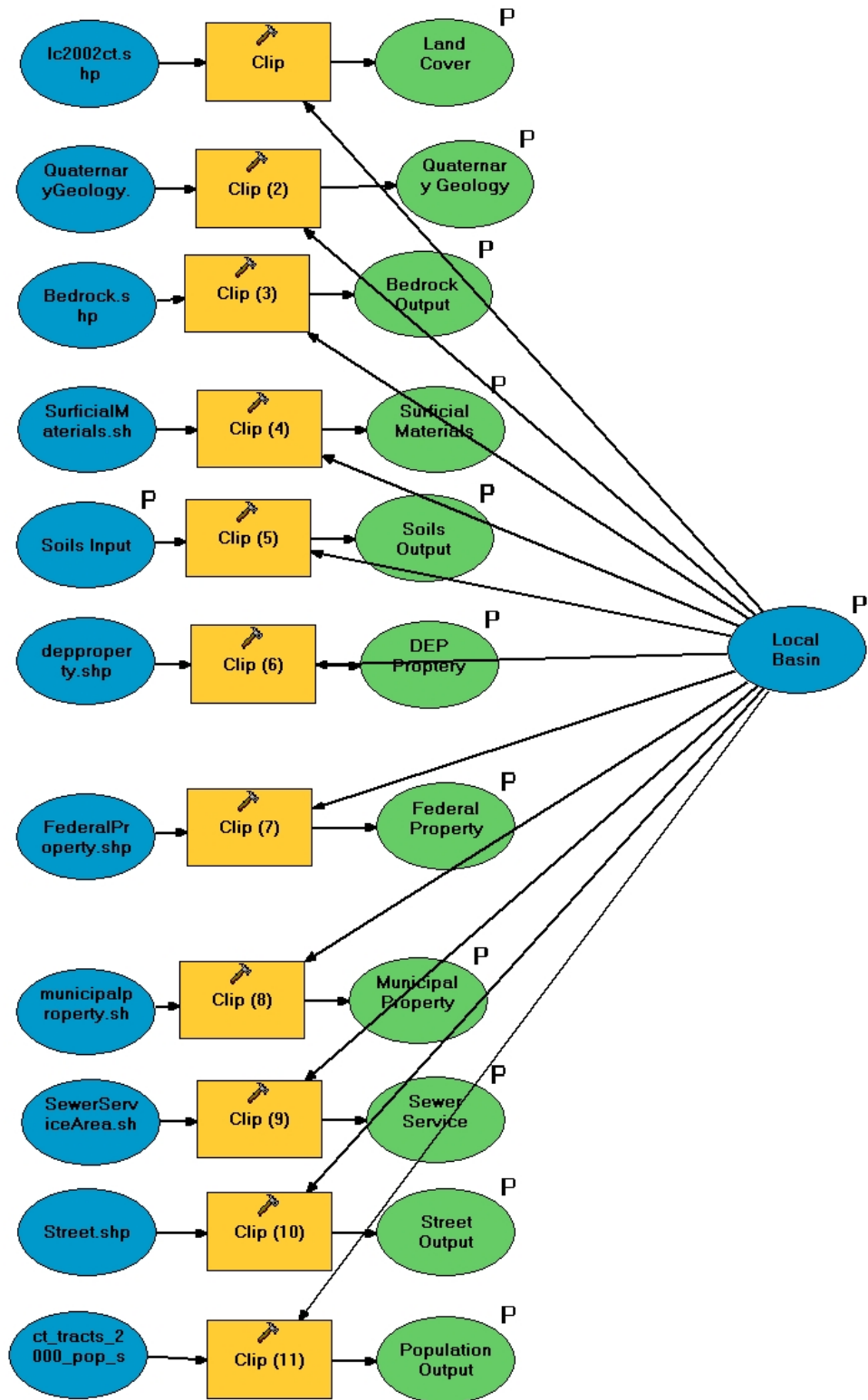
Figure 3: Schematic of the clip model, which was used in ArcView to clip various shapefiles to the desired basin.
