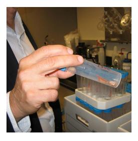
Dried, ground plant material in test tube waiting for testing in an inductively coupled plasma mass spectrometer (ICPMS). It can determine whether the elements in question are present and in what volume.
