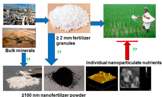
Figure 1. Conceptual overview of fertilizer advancement from bulk-scale to nanoscale production and application. The question marks represent some of the open questions such as scaling up production and safe and effective nanofertilizer application methods. The blocked (red) arrow indicates that this representation does not advocate for the broadcast application of nanofertilizers.
