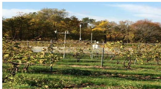
Figure 8. Anemometers measure wind information in a Pinot gris vineyard at Lockwood Farm in Hamden CT.
