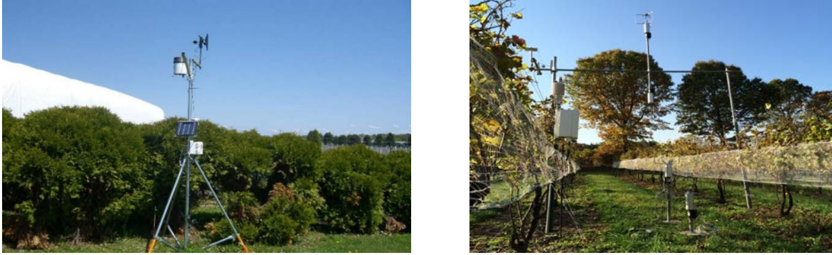
Figure 2. 3D-sonic anemometers measure wind data in a Pinot Gris vineyard at Lockwood Farm.
