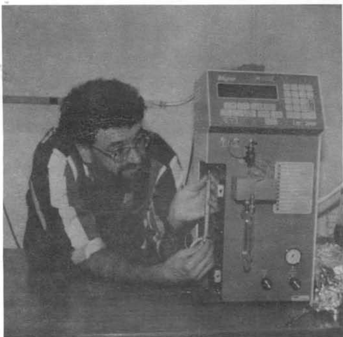
Figure 1. Brian D. Eitzer placing a sorbent resin tube into the thermal desorption oven of a gas chromatography/mass spectroscopy instrument.
