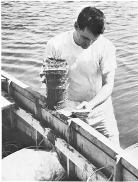
This plastic cylinder, a core sampler, is pushed into the mud. Then the sample is subdivided by plastic blades to keep larvae in sub-samples of known depth.
