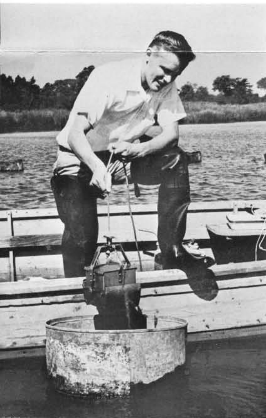
Dr. Anderson dredges a sample of mud from a bottomless drum used to make a test area for insecticide studies.
