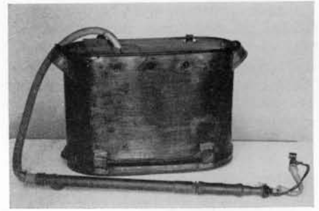
A homemade sprayer used by Thaxter in 1888. The tank is a small copper washboiler.
