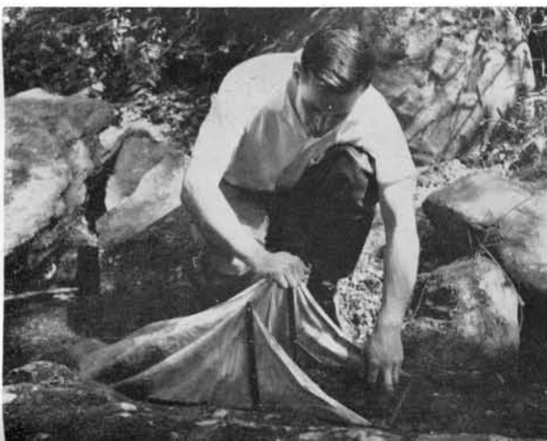
Dr. Hitchcock collects underwater insects in a foot-square Surber sampler, transfers them to tray for study.
