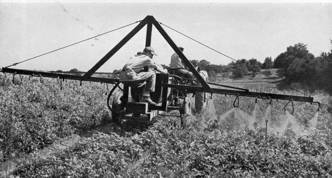
Experimental sprayer for small plots of potatoes. Miss Nancy Woodruff, the spray operator, opens a valve on the side to be sprayed. Plots are usually 15 to 25 feet long and 3 feet wide. Materials that perform well on small plots are then taken to commercial fields for large scale tests.
