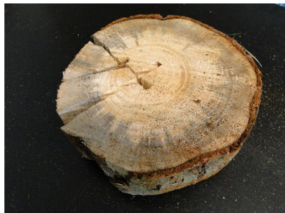
Figure 2. Sectors of blue discoloration in pine log, caused by blue-stain fungi.
