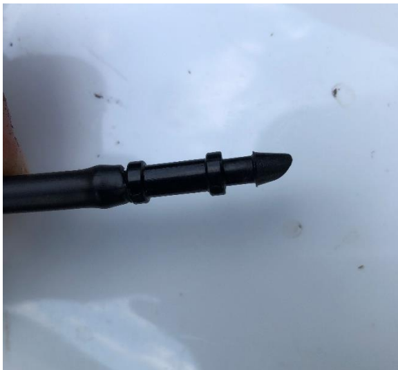
Figure 9. Close up of the 1/4" barb connector on the end of the leader.
