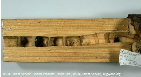
Fig. 2: Carpenter bee gallery and brood cells
