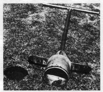
Fig. 2. Core sampler used in examining soil for Japanese beetle grubs; diam.  $\pm$  6.4 inches.
