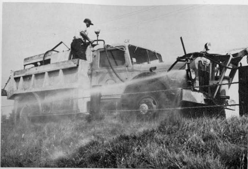
Figure 1. Application equipment shown above is one of the types used for control of broadleafed weeds in roadside turf and for the control of low brush with foliage sprays.
