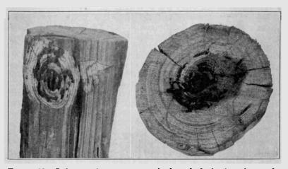
FIGURE 92. Left: section cut at an angle through the laminated part of a carpenter ant cavity in a telephone pole. Right: cross section through a treated ant cavity below the level at which the creosote was applied. The dark stain is due to creosote.
