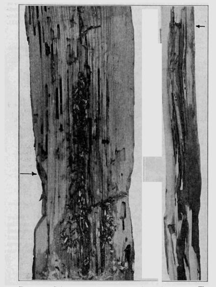
FIGURE 91. Left: carpenter ant colony in telephone pole in winter. The arrow indicates the ground level. The section is about 2 feet long. Right: longitudinal section of a treated pole. The dark stain is due to creosote injected at the level indicated by the arrow. The section is about 4 feet long.
