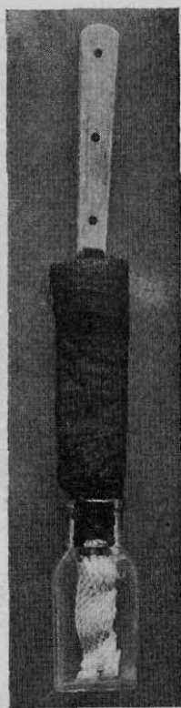
FIGURE 105. Sheath to hold knife. Two flat lamp wicks sewed together at their edges and covered with tape, the lower end immersed in alcohol, keep the knife blade sterile.
