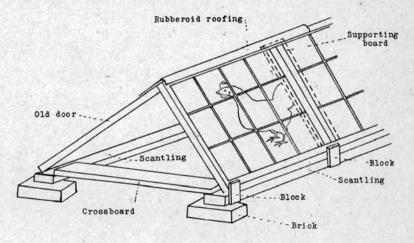
Before putting the sashes in place the doors were supported at the proper angle by boards about six inches wide which were nailed to the scantling at the lower end and to the door at the upper end. These boards were so placed that the ends of adjacent sashes rested on them when in place and in this way rain was prevented from running into the cracks between the sashes.
