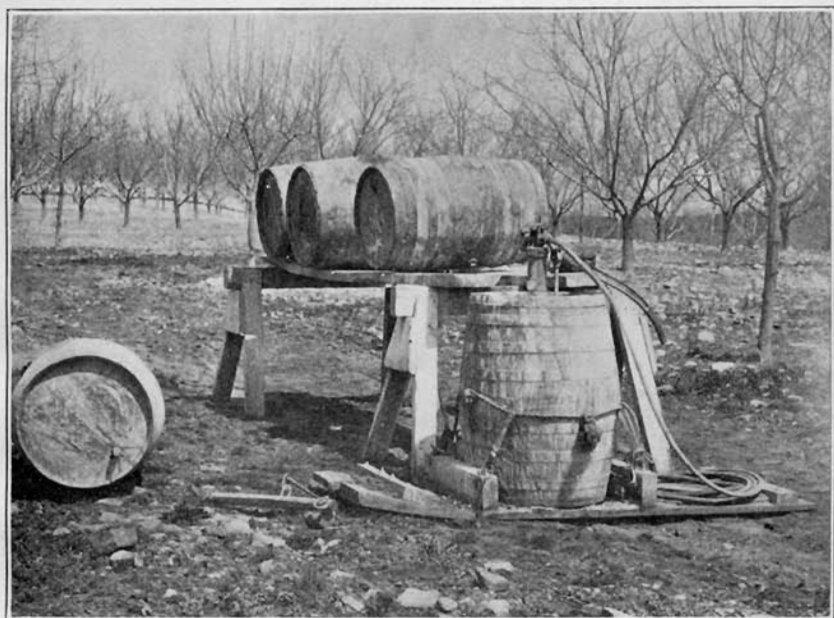
b. View in Barnes Brothers' orchards showing elevated storage barrels and spraying barrel and pump mounted on stone drag.
