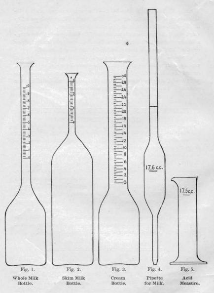
graduated from 0 to 30 (figure 3). The graduated portion of the neck is about the same length as that of the whole milk bottles, but has three times its capacity. The divisions of the scale represent 0.5 per cent., but can be read to a quarter of a division.
