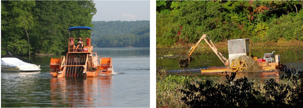
Figure 15. Cut and capture harvesting machine in Lake Zoar, CT (left). Hydroraking machine in Lake Quonnipaug, Guilford, CT (right).
