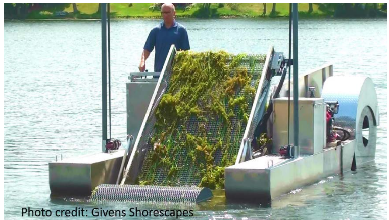
Figure 10. Eco-Harvester technology may improve removal of plant roots.
