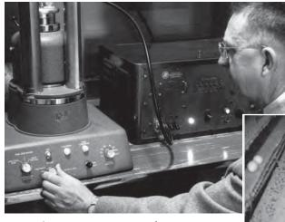
Figure 43. Dr. Raimon L. Beard, using a Thin-Window Counter (early radiation detector), 1961.
