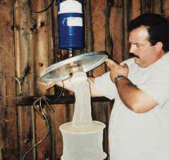
Figure 31. Michael Vasil examines a CDC light trap for mosquitoes, which uses carbon dioxide as well as a light to attract mosquitoes. A fan draws the mosquitoes down into the netted cage, 2000.
