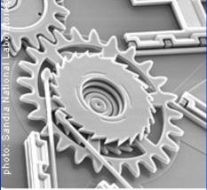
This nano-machine is 50 microns across and can only be viewed using a powerful Scanning Electron Microscope. For comparison, a human hair is about 100 microns across.
