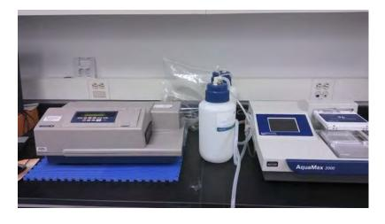
Spectramax M5 and Aqua Max plate washer
