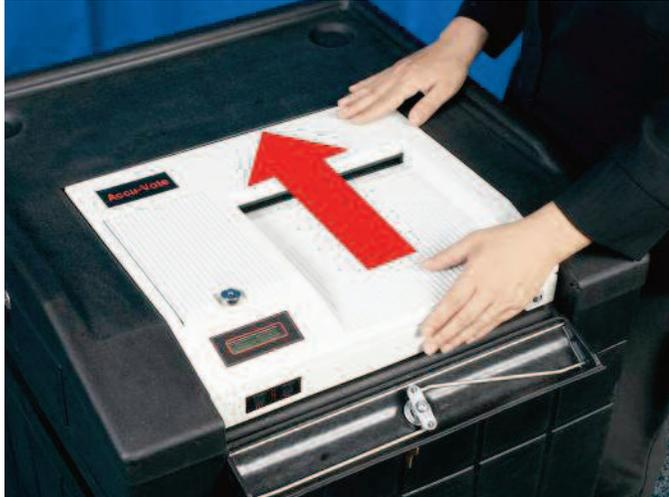
Step 19 – Slide the Optical Scan unit all the way back until securely seated
