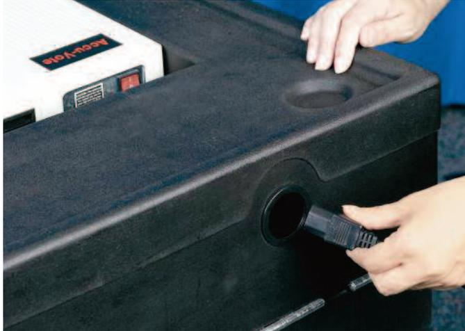
Step 9 – Feed the power cord through the tunnel in the back of the ballot box
