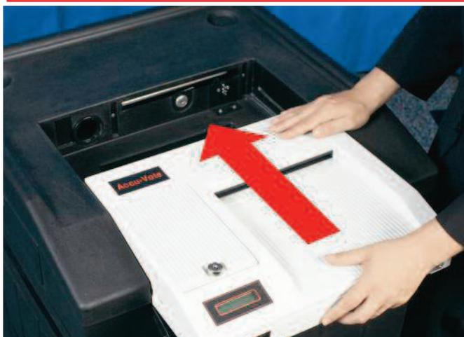
Step 8 – Slide the Optical Scan halfway into the ballot box
