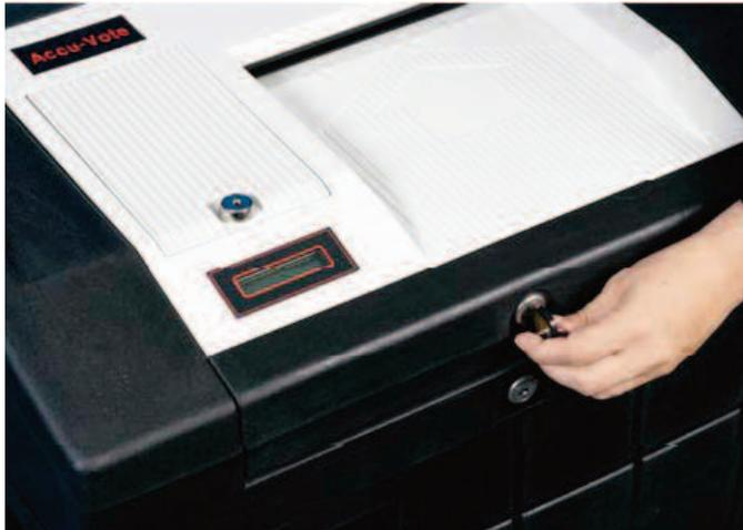
Step 20 – Close and lock retaining door
