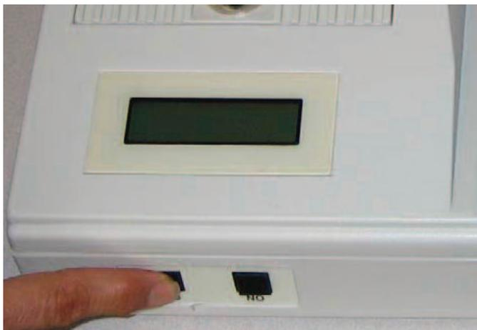
Step 4 – Override overvote rejections by holding the YES button and feeding the ballot
