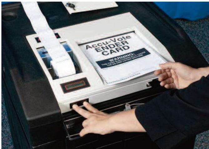
Step 9 – Feed Ender Card while pressing and holding the YES and NO buttons
