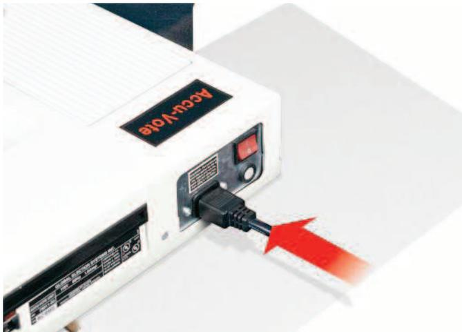
Step 10 – Plug the female end of the power cord into the Optical Scan unit
