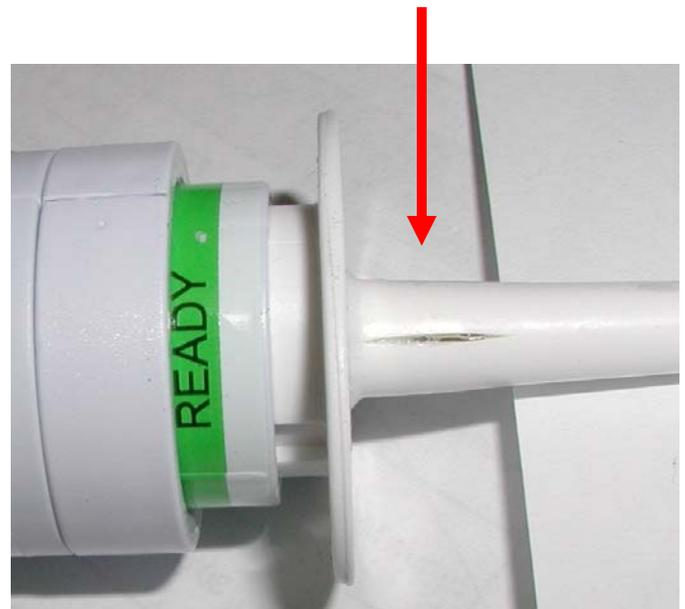
**Example of a Crack at the Base of the Syringe Tip**
