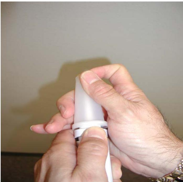
Step 4: While maintaining pressure on the seal pin apply an upward force to close the cap. Rotate the syringe 180 degrees and repeat steps 3 and 4.
