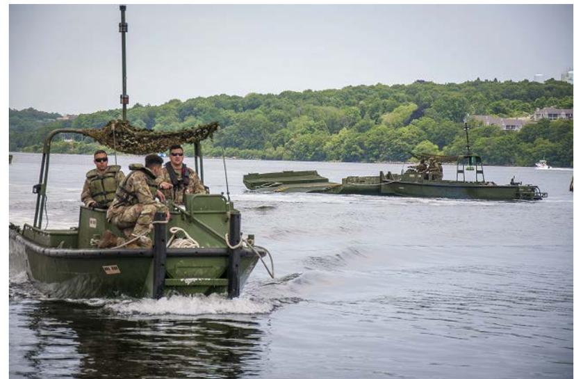
A team from the Connecticut National Guard's 250th Multi-Role Bridge Company drives their Bridge Erection Boat back toward the shore after dropping off a segment of an Improved Ribbon Bridge on the Thames River, June 10, 2020. The IRB team practiced creating a five-float raft which is designed to transport troops, equipment, and vehicles across a river. (U.S. Army photo by Tim Koster, Connecticut National Guard Joint Force Headquarters Public Affairs)
