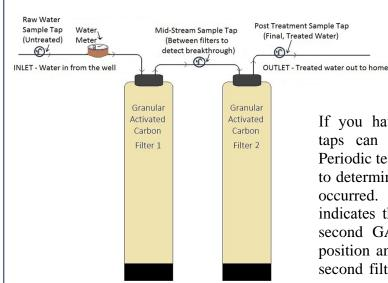
If you have two GAC filters installed in series, sample taps can be installed pre, mid and post GAC filtration. Periodic testing can be performed pre, mid and post filtration to determine when service is needed or if breakthrough has occurred. Once the mid-stream water quality sample indicates that the GAC filter media should be changed, the second GAC filter is often times swapped to the front position and a filter with new GAC media is moved to the second filter position.
