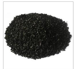
GAC maintenance frequency will vary based on the size of the filter unit, household water usage, contaminant concentration levels, and overall water quality. Water quality testing can help determine when GAC media needs to be replaced. A water meter installed at the filter may be helpful in determining when carbon replacement is necessary. Refer to the two sections below for more information.
