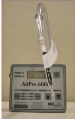
Air contaminants stick to media in a solid sorbent tube after air is drawn through with a pump. Analysis occurs in the lab.
