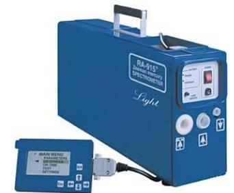
Special portable direct reading instruments like this one provide instant mercury vapor results.
