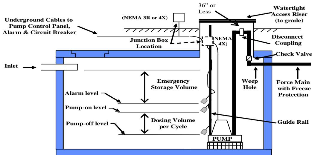
**Figure 11 - Pump Chamber**
