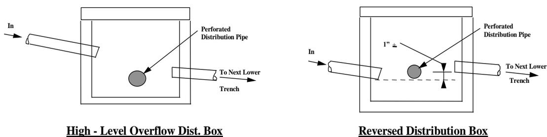
The high-level overflow invert elevation shall be set within the top 3 inches of the upper leaching system row. In order to ensure adequate gas transfer, the use of reversed distribution boxes should be avoided.
