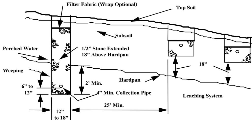
**Figure 17 - Typical Curtain Drain Construction**
