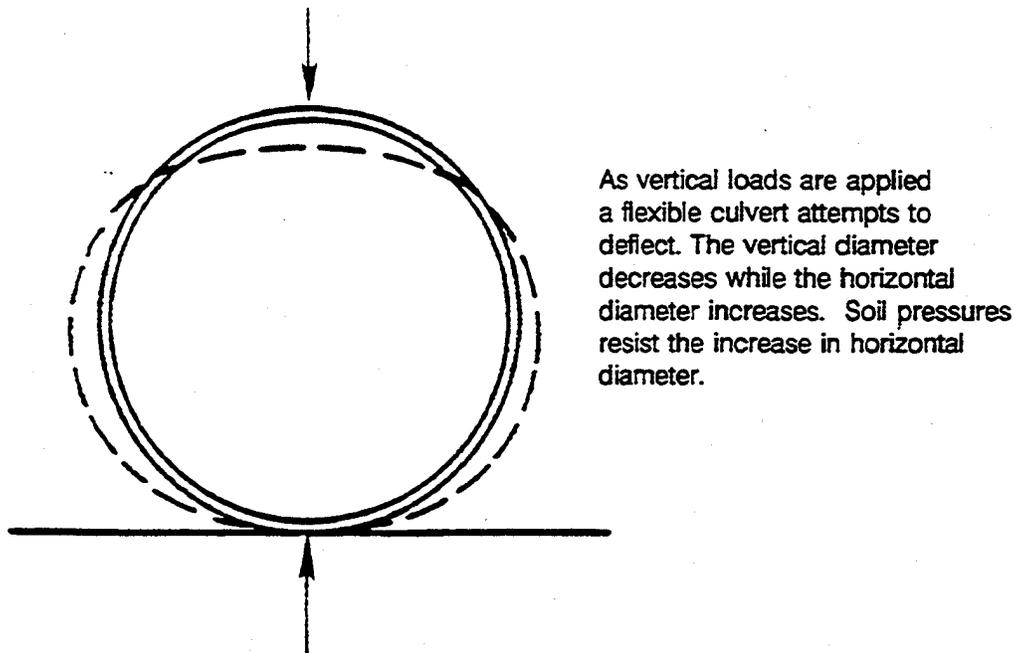
**Figure 4-4 Deflection of flexible culverts.**
