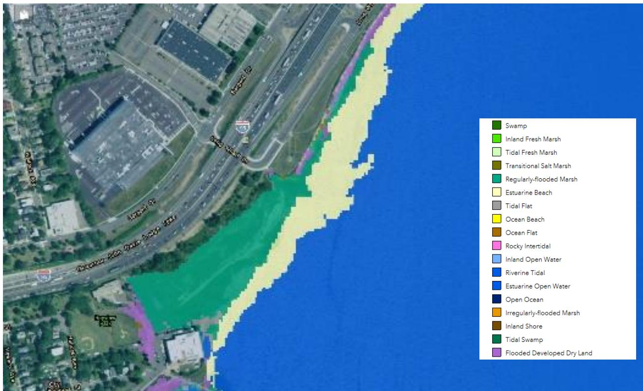
**Figure 4-2: Connecticut SLAMM Model +/- 2.5 feet Sea Level Rise**
