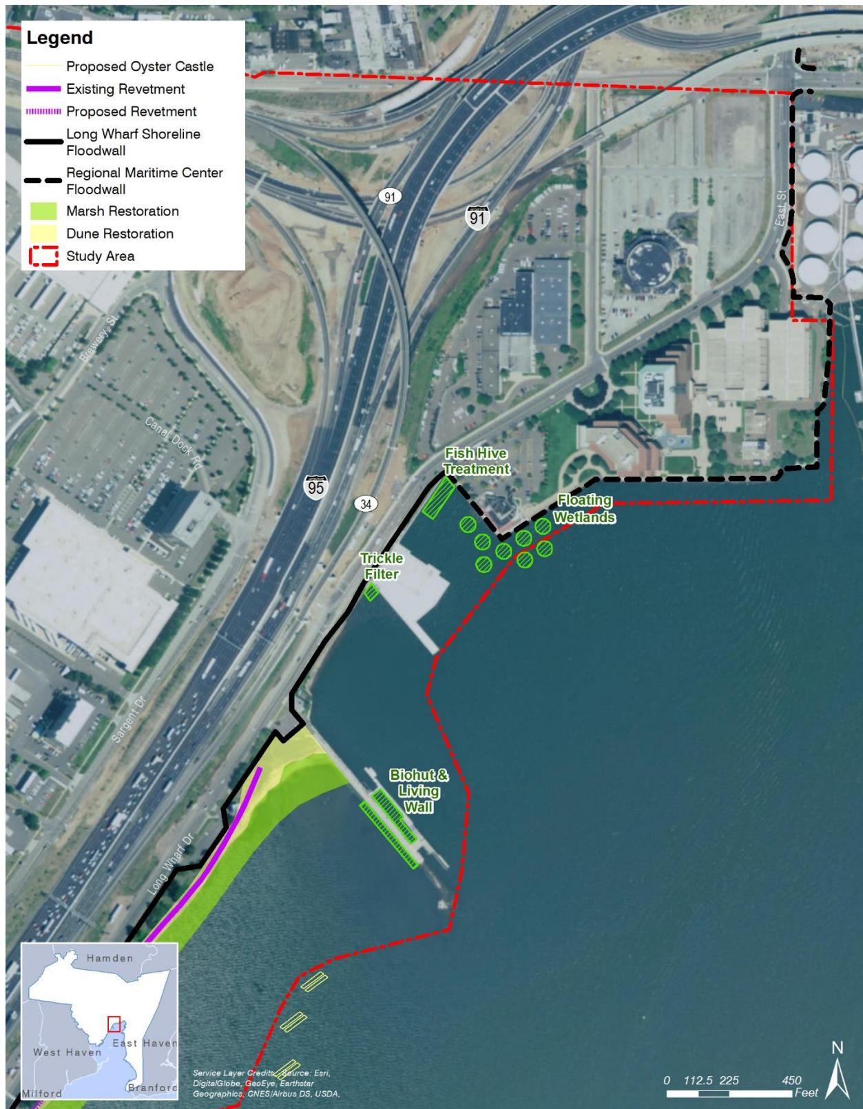
**Figure 6-1: Alternative 4 Concept Drawing showing Project Components (North)**
