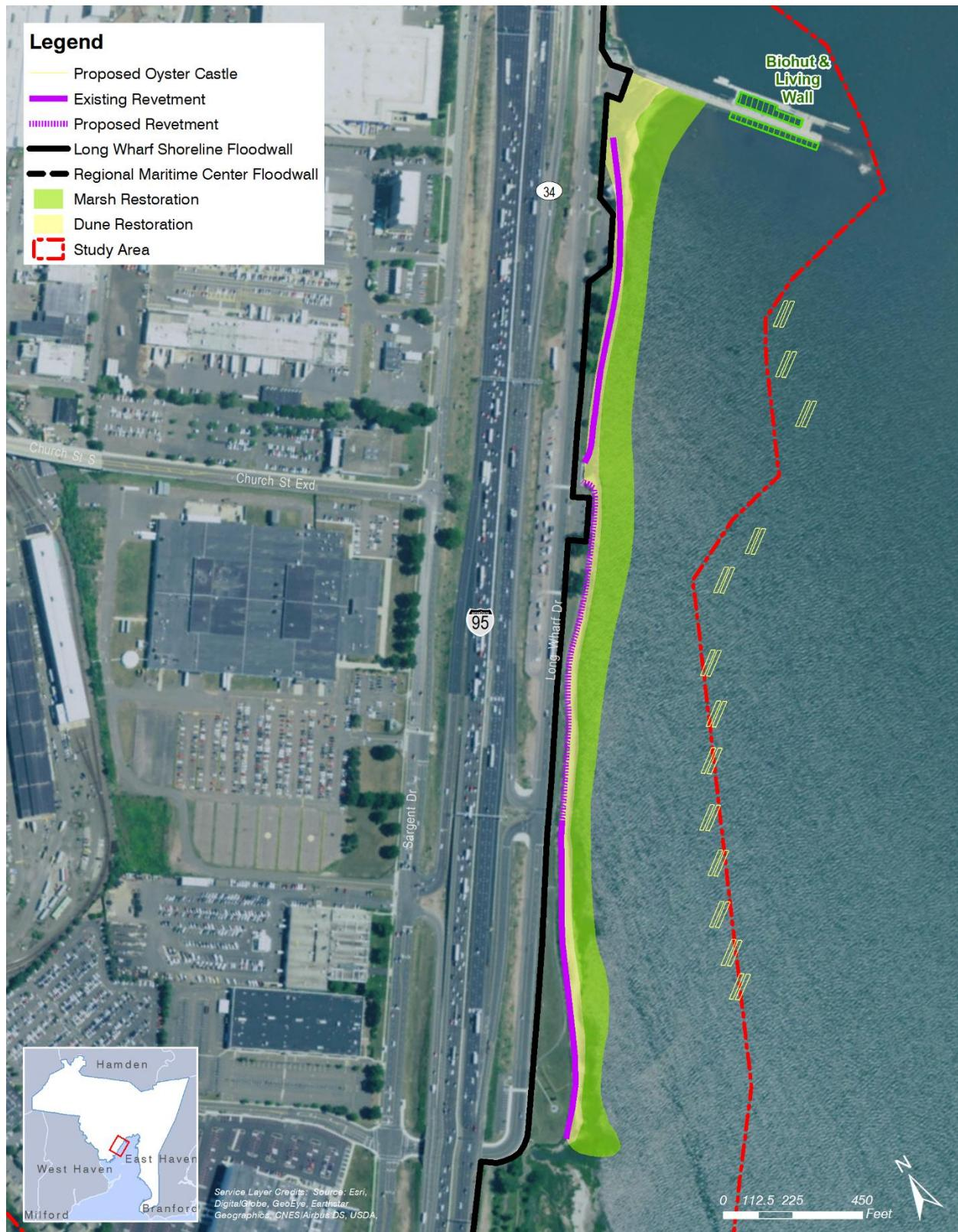
**Figure 6-2: Alternative 4 Concept Drawing showing Project Components (Middle)**
