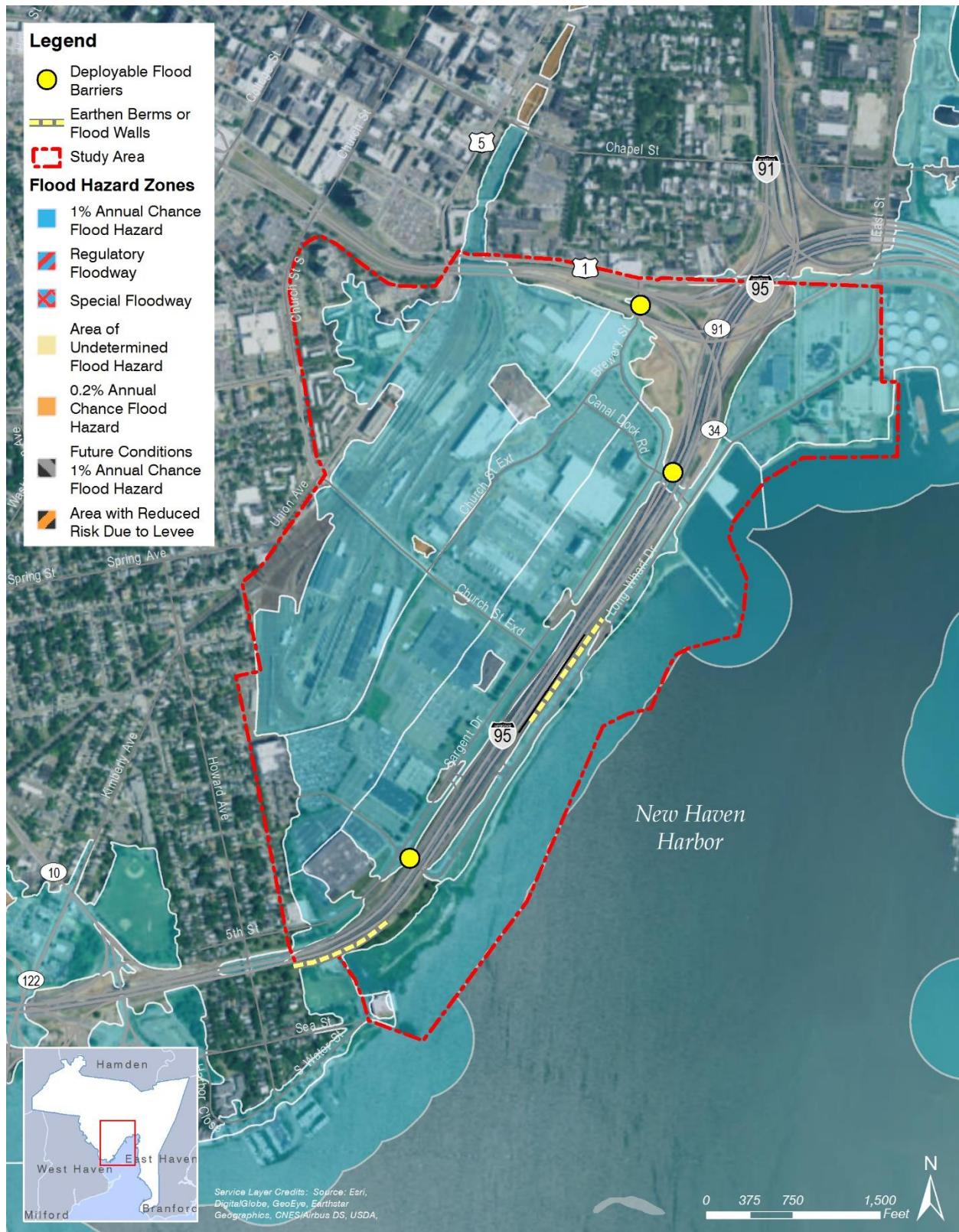
Figure 1: Location of Proposed Deployable Flood Barriers (FEMA Flood Hazard area shown)
