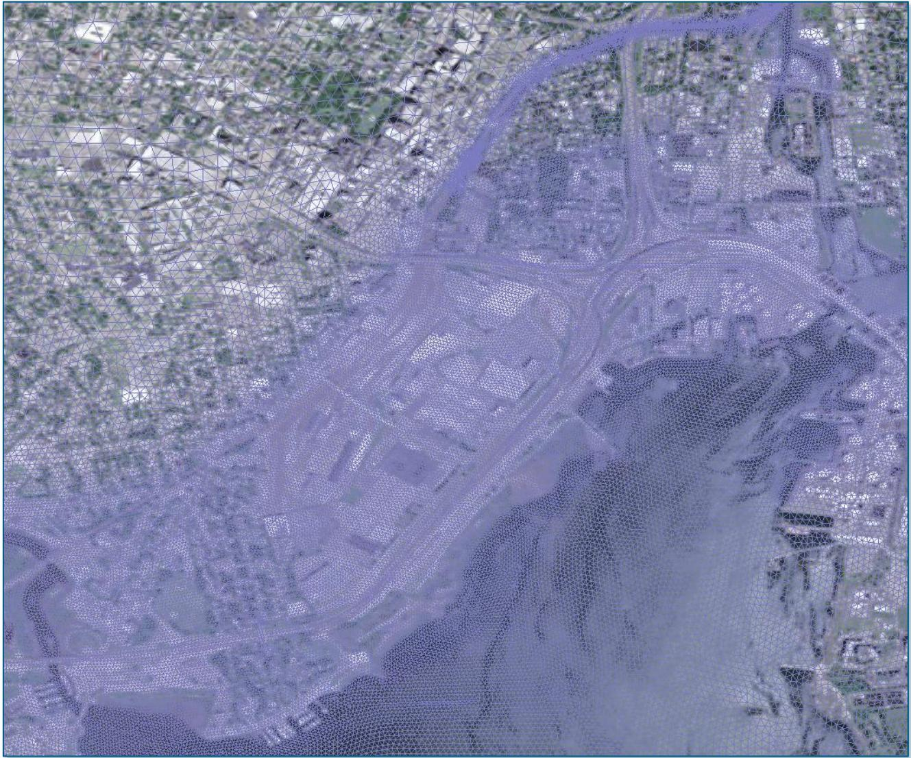
**Figure 3-18: High Resolution Mesh Used for Flood Model Simulations at Long Wharf**
