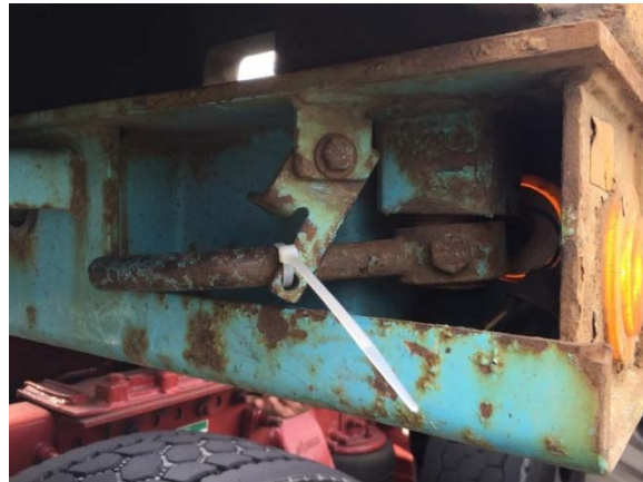
Figure 4: Use of Additional Tie-wrap
