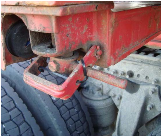
Figure 4: Use of Additional Tie-wrap
