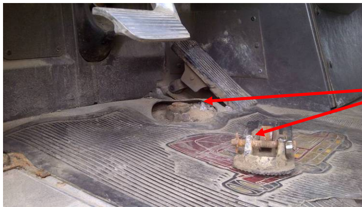
Figure 1: A detached brake treadle illustrates a potential result of excessive corrosion damage.
